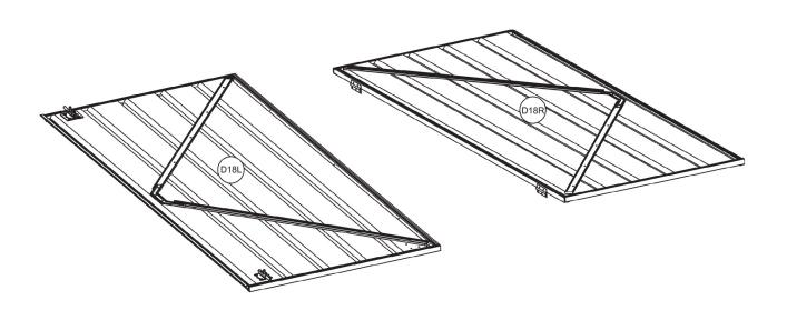
Fit parts D18L and D18R (assembled doors) to the front wall panel as per the diagram below. Use rivet gun and pre-drilled holes. Fix parts 70 (pad bolt) and 71 (keeper) to the doors using the pre-drilled holes and 16mm self-tapping screws (or the rivets provided - see diagrams A and B).
