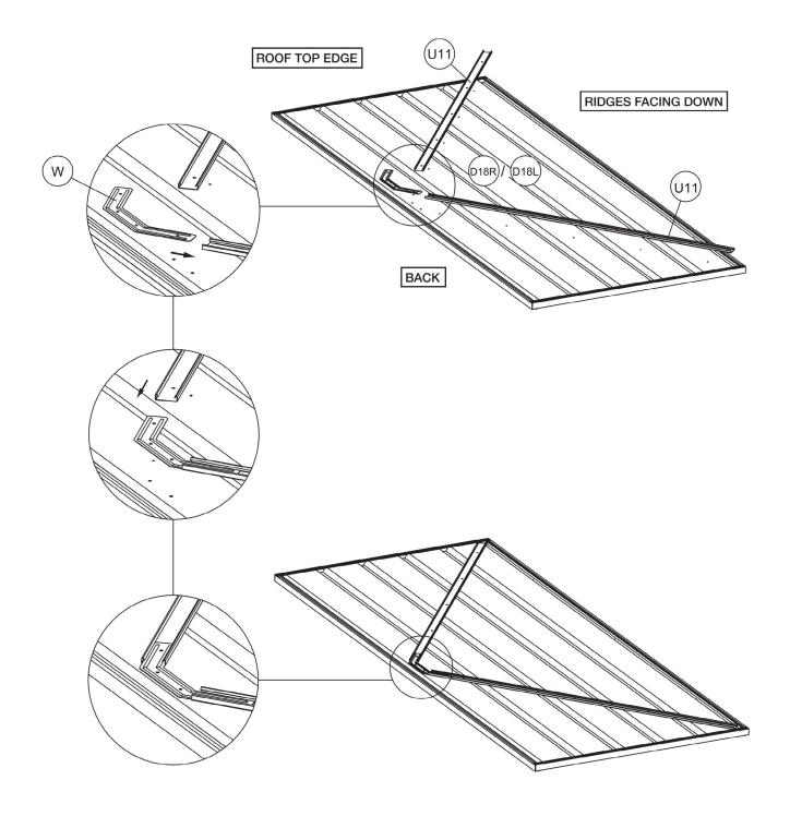
Turn door over with bracing still aligned with holes (make sure the ridges of the door are facing up) and fix the bracing with 3.0 x 10mm rivets through the front of the panel. Then turn door over and insert plastic stoppers at the ends of braces as shown below.
