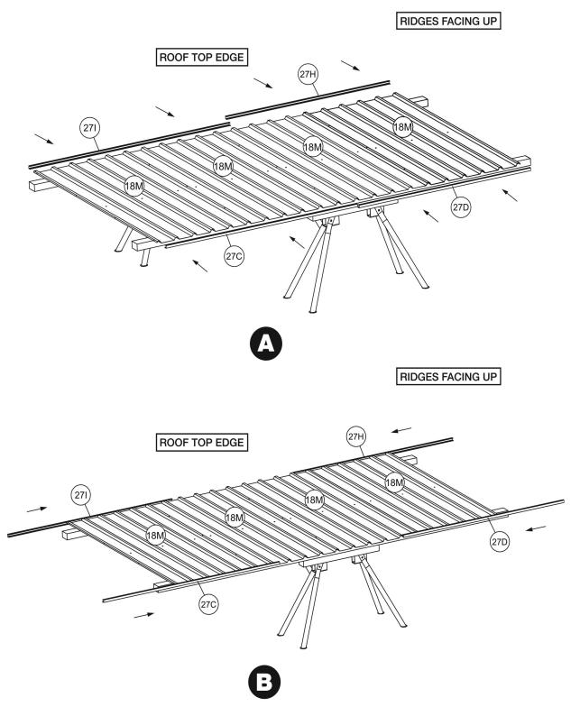
Tip: If panel and screw holes do not line up, try pulling panel to match up holes.
